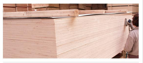
Fireply is a lightweight, fire-retardant plywood ideal for interior cladding use in commercial and residential buildings.
